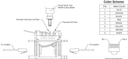
IC06628P8C Prewired 66-Block with 12 RJ-45 8P8C Jacks
