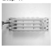
1. Mount the IC110 hinged wiring block onto an appropriate surface with the included mounting screws or any other necessary hardware.
